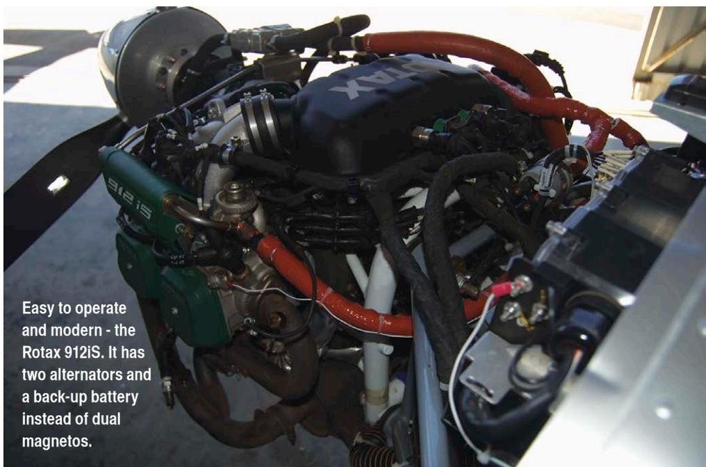
**Easy to operate and modern - the Rotax 912iS. It has two alternators and a back-up battery instead of dual magnetos.**
